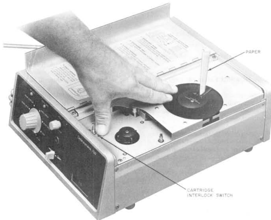
Fig. 7—Resetting "0" Registration on Message Indicator Dial
