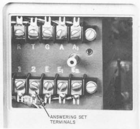
Fig. 27—KS-19245, List 1 (MD) Telephone Answering Set—Terminal Board
