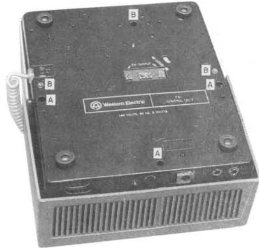
A - REAR HOUSING ASSY CAPTIVE SCREW ACCESS HOLES B - MICROPHONE AND FRONT HOUSING ASSY SCREWS AND CAPTIVE SCREW ACCESS HOLE
